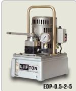
**EDP-1 Series** electric pump are available with 3 or 4 way Solenoid and manual valves. Models are available on 220/240V Single Phase and 380V three phase. The two stage pump switch over from low pressure to high pressure at 70bar pressure. Most commonly used with Lifton single acting and double acting cylinders.
