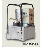
**EDP-3 Series** electric pump are available with 3 or 4 way solenoid and manual valves. Models are available on 380V three phase. The two stage pump switch over from low pressure to high pressure at 70bar pressure. These are heavy duty pumps with very high flow at high pressure and widely used where quick operation is required under load.
