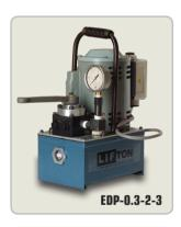
EDP-0.3 Series electric pump are available with 3 or 4 way solenoid and manual valves. Models are available on 220/240V single phase .The two stage pump switch over from low pressure to high pressure at 50bar pressure. Most commonly used with Lifton cylinders with small strokes and also with single acting hydraulic tools.
